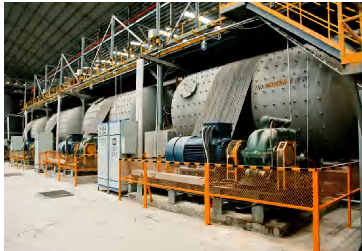
连续球磨机 | Modulos Continuous Ball Mill
